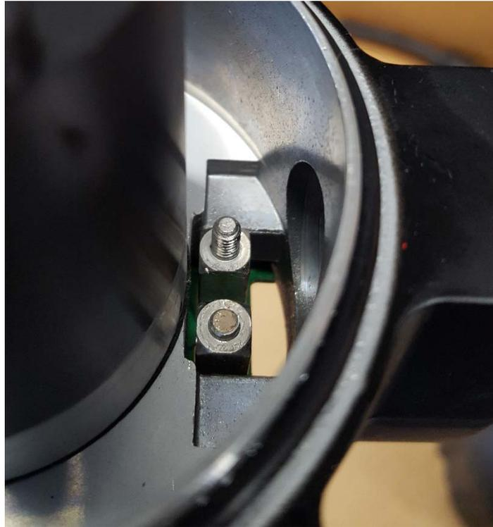
Figure 11: The sheared terminal stud of the second thruster
