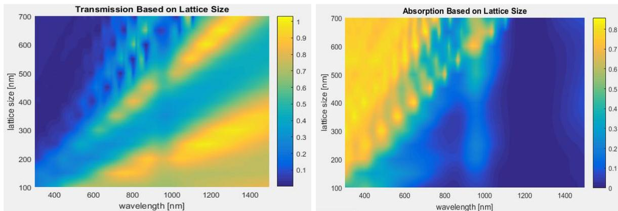
(Fig. 4 (a)) Transmission of the CQD-based cell as the film thickness, spacing, and inclusion diameter increase proportionally
