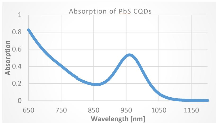
(Fig. 3) Absorption spectrum of CQDs synthesized in the lab
