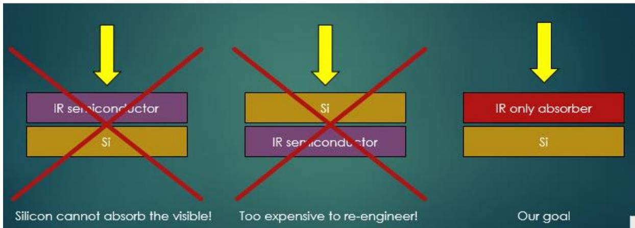
(Fig. 2) Various tandem solar cell designs
