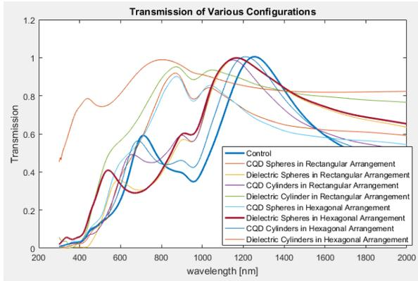
(Fig. 5 (a)) Transmission of the CQD-based cell with various inclusion shapes and material in hexagonal and rectangular arrangements
