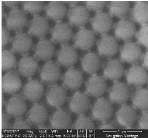
(Fig. 6) A Scanning Electron Microscope (SEM) image of polystyrene bead in hexagonal formation
