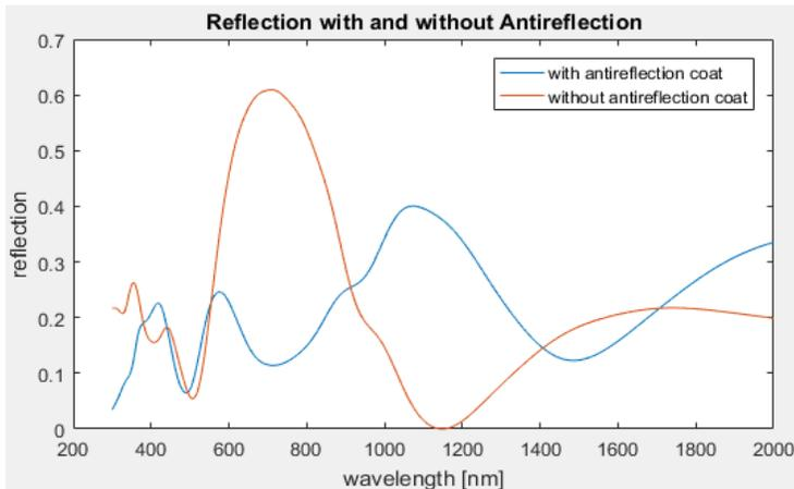
(Fig. 8) Reflection of the CQD-based cell with 250 nm dielectric spherical inclusions within a 250 nm thick CQD film and a 140 nm AZO / 100 nm MoO<sub>3</sub> antireflective coating compared to the control of the 250 nm dielectric spherical inclusions within a 250 nm thick CQD film without any antireflective coatings.
