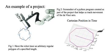
From this we realized that we needed to create an easy to use API for these students to move the robot around with. The da Vinci surgical machine uses both Cartesian movement and joint movement. Therefore, we gave them choices to move in both Cartesian space and joint space. We also decided to give them a choice of incremental motion, as well as absolute move. We also created other methods for easy control of the surgical robot. From this we created the following API:
